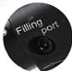
Hydraulic oil adding port
